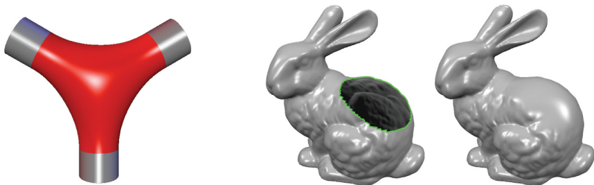
Figure 4.7. Applications of surface fairing include constructing smooth blends between given surface parts (left) and filling holes with smooth patches (right).
